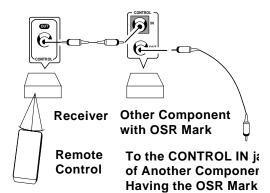
If you also have an Optimus professional series CD player, VCR, or cassette deck with the OSR mark, you can connect its **CONTROL IN** jack to the receiver so you can control all of your equipment with a single remote control. You can also use the other component's remote control by pointing it at the receiver's front panel.
